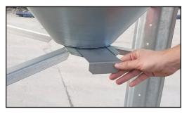
MBSLGT and MBSLGT+20 come with a slide gate for feed discharge at the bottom of the cone (see above). These bins cannot be used with rigid or flex auger.
